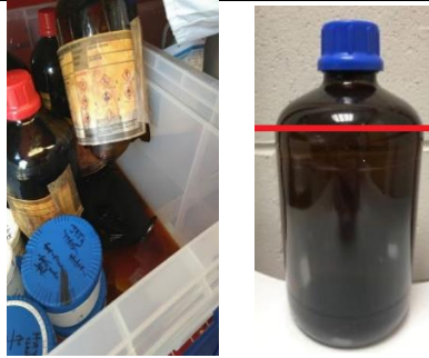
Figure 1 – Example of an incorrectly used Winchester and guide fill point
