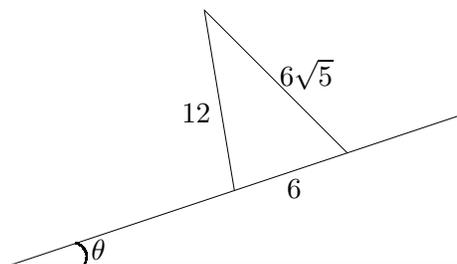
Assuming that the coefficient of friction is such that the prism does not slide down the slope, show that the largest value of  $\theta$  for which the prism will not topple over satisfies,
