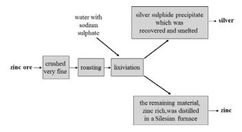
Fig. 6 A suggested flow diagram for the 'special process' used by Dillwyn & Co.
