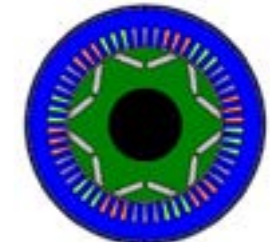
Model 3 motor design on Pyleecan
